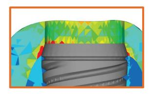
From the simulation results, it can be concluded, that – because of the relatively low and evenly distributed stresses in the cortical bone – the examined thread formation is advantageous in respect of the normal function of the healed implant, compared to those conventional screw implants, which possess smooth surface in the cortical bone region.
